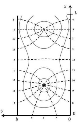
15. The above figure depicts an idealized solution for the expected propagation of tidal waves in a semi-enclosed rectangular basin of uniform depth, with dashed lines representing places with the same tidal phase at a given hour (cotidal lines). A system exhibiting the motion above could theoretically be found in which of the following regions?
