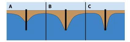
The figure above shows three wells surrounded by cones of depression, regions where overpumping of groundwater has occurred. Which of the following statements correctly describe the environments of wells A, B, and C?
